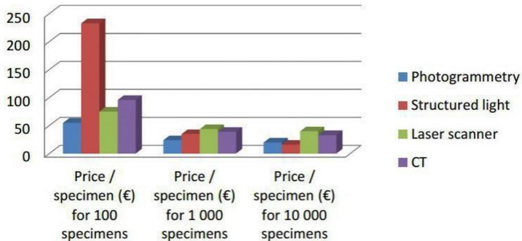
Graph 1: Cost of the digitisation of 1 middle sized specimen in function of the technique and of the quantity of specimens to be digitised. The cost takes into account the equipment, time of digitisation and salary of the staff.
